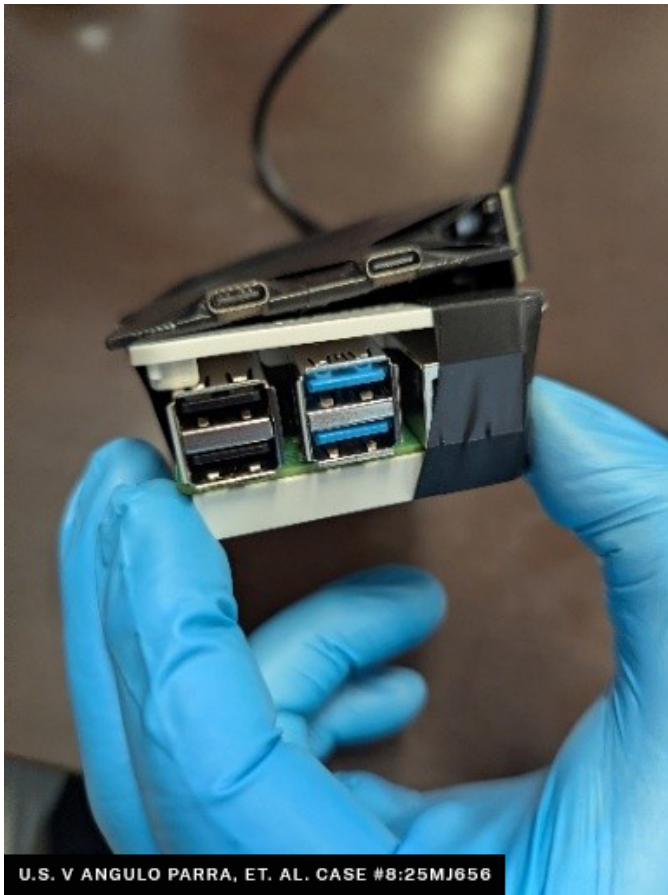
Fig. 2. A modified hardware device recovered by law enforcement, used to inject malware into the ATM’s internal PC.
