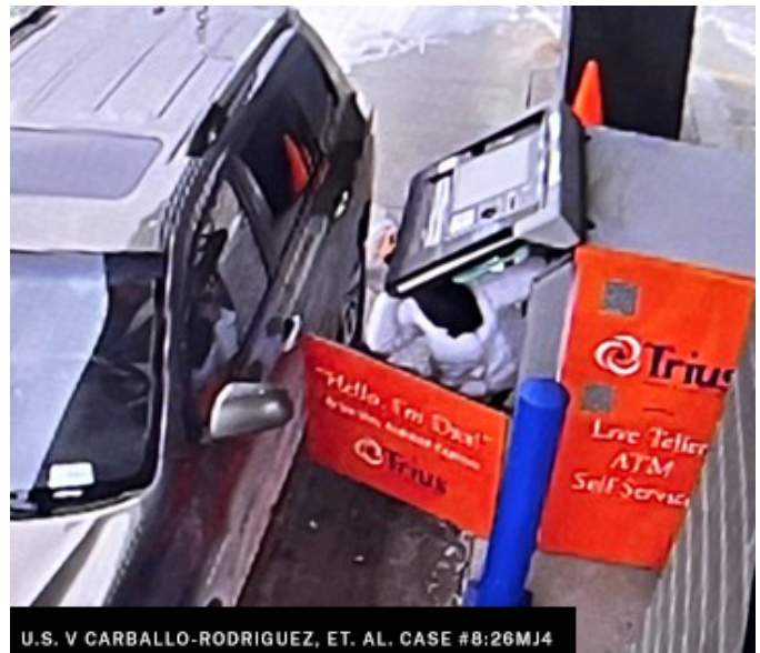
Fig. 1. Surveillance footage of a physical intrusion into an ATM cabinet during a jackpotting attack.
